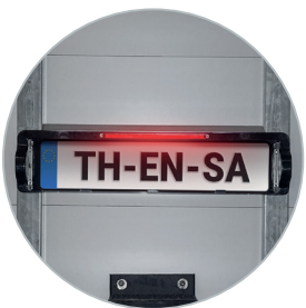
Third brake light LED in licence plate holder
