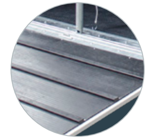
Low entrance tailgate ramp with rubber top, cross step bars and side stops
