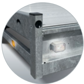
LED marker lights at the front
