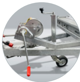
Accessorie: Adjustable winch support for left- and righthand use
