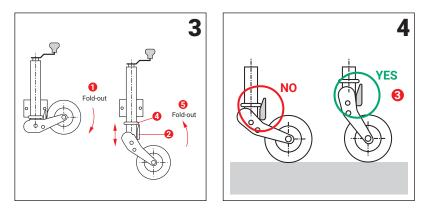
When rotating the nose wheel, make sure that the brake rod of the trailer remains free of any part of the nose wheel. If the brake rod comes into contact with the trailer, optimum braking is no longer possible.
