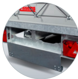
Standard equipped with integrated ramp holders
