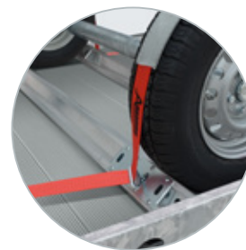
Accessorie: Wheelstop and Easyfix straps
