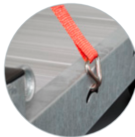
Recesses for tie-down possibilities
