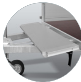
Front-panel can rest on the A-frame
