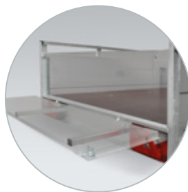
Back-panel can rest on pullout beams
