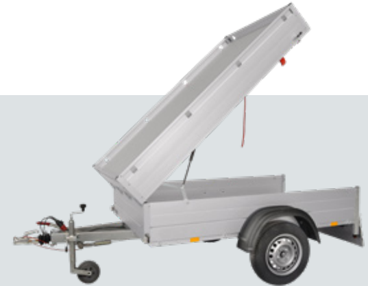
GT-HT single-axle braked (internal height 48 cm)
