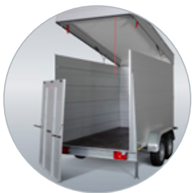
The aluminium tailgate ramp is easily removable
