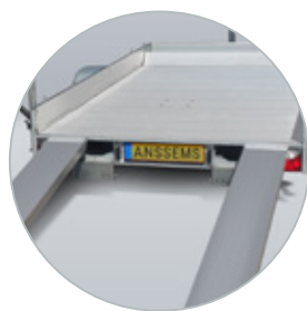
Aluminium ramps in integrated ramp holders
