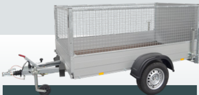
Mesh sides with a height of 70cm will increase the load capacity. Ideal for transporting bulk goods. This picture shows the GT-O in combination with a tailgate ramp and propstands.
