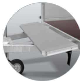
Front-panel can rest on the A-frame
