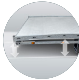
Lowered load floor at rear
